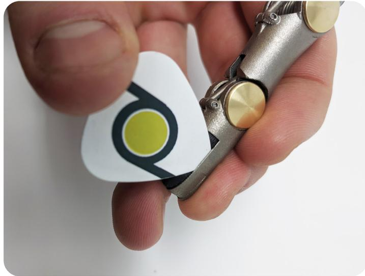
**3.** With the edges pressed in, apply pressure to the top of the pad and rock back and forth gently to help make sure the pad is fully seated. If the pad looks to be bulging out still, then repeat Step 2.
